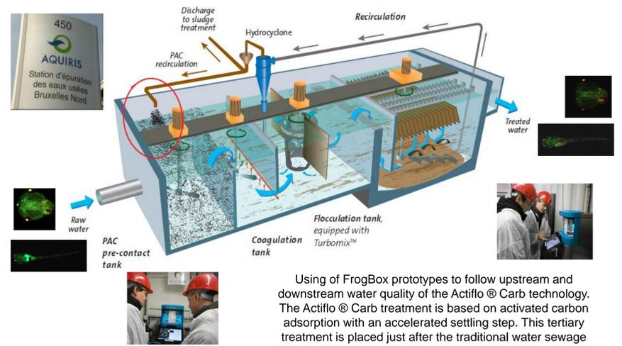
Using of FrogBox prototypes to follow upstream and downstream water quality of the Actiflo® Carb technology. The Actiflo® Carb treatment is based on activated carbon adsorption with an accelerated settling step. This tertiary treatment is placed just after the traditional water sewage plant treatment
