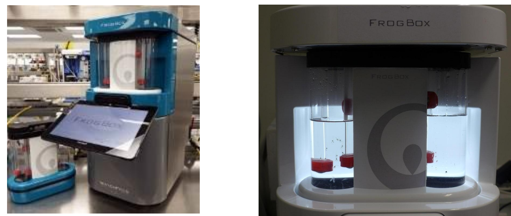
The FrogBox (left). Tadpole swimming into the larvae cartridge in "day" mode (right)
